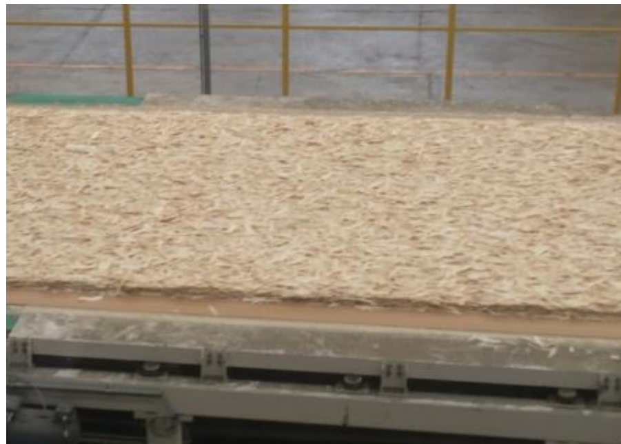
Fig. 7 Example of the third layer for OSB prior to press infeed
