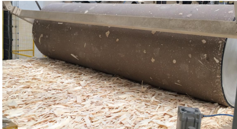
Fig 6 Levelling and compressing the two outer layers for the OSB board
