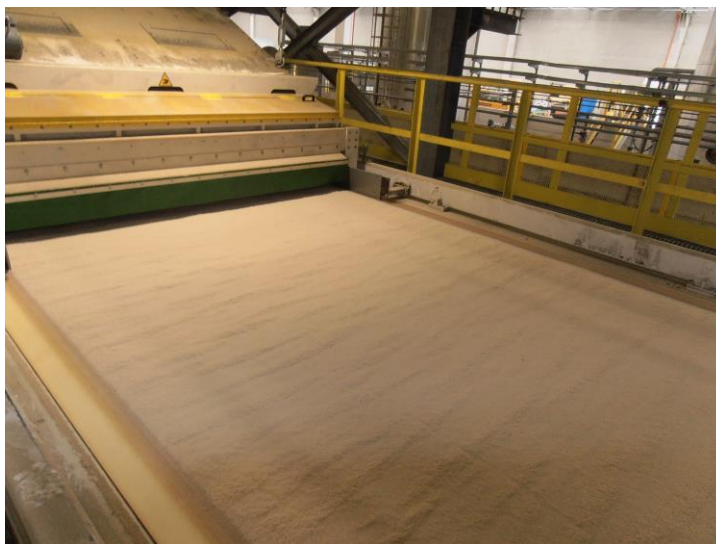
Fig. 1 forming of the wood dust layer for the production of the LSB panel
