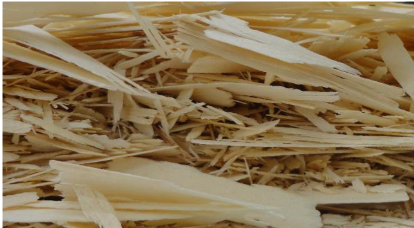
Fig.4 Strands after the drying process
