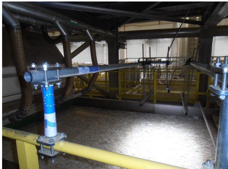
Fig. 13 example of the optical system on the first OSB layer
