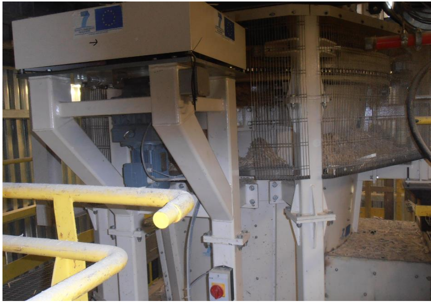
Fig.8 cone-shaped rotary chute
