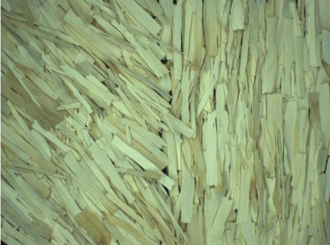
*Figure 14 An image from validation dataset, having a predetermined orientation distribution. The strands in the right part of the image are oriented according to a 90° angle, while in the left part the orientation is 135°.*
