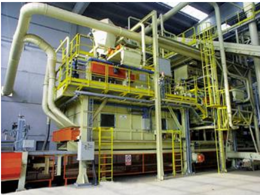
Figure 4 – Face layer wind forming system. Partial view of the complete particle mat forming system
