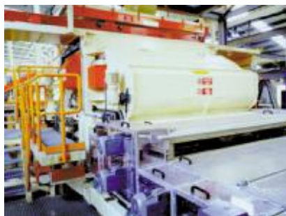
Figure 6 – Face layer CrownFormer. Partial view of the complete particle mat forming system
