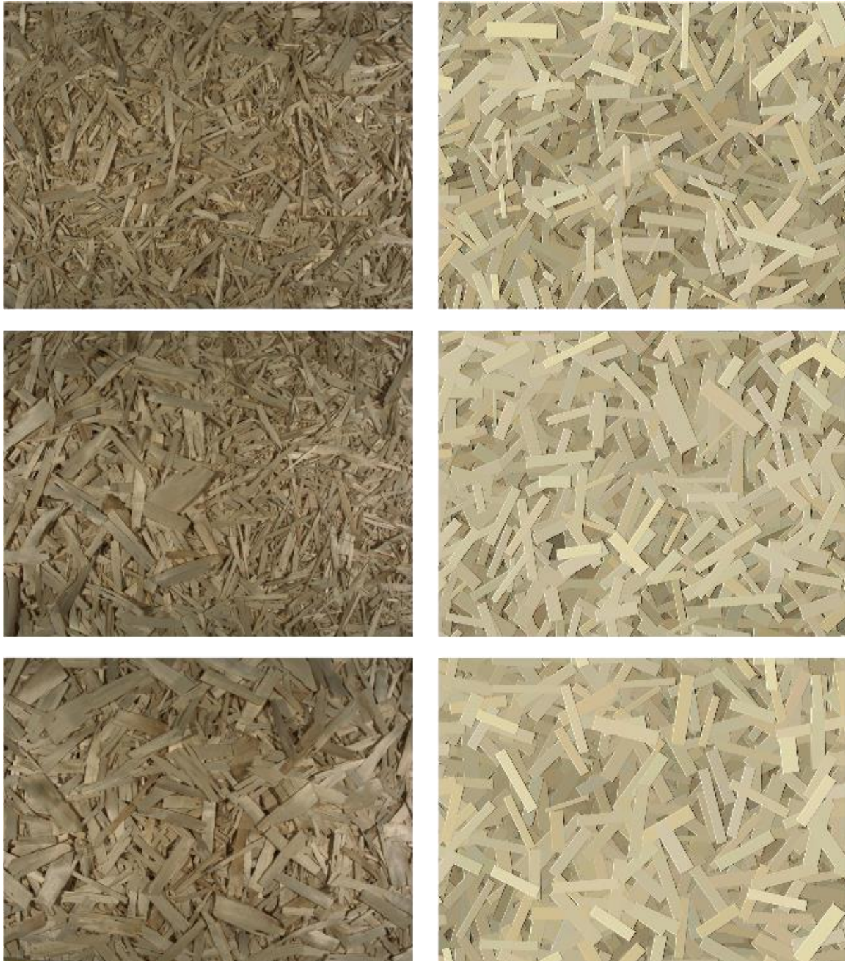
Figure 25 - Examples of the images used in the tests. First column shows images of the real mattress, second column presents synthetic images. The size of the strands present in the images increases from top to bottom.
