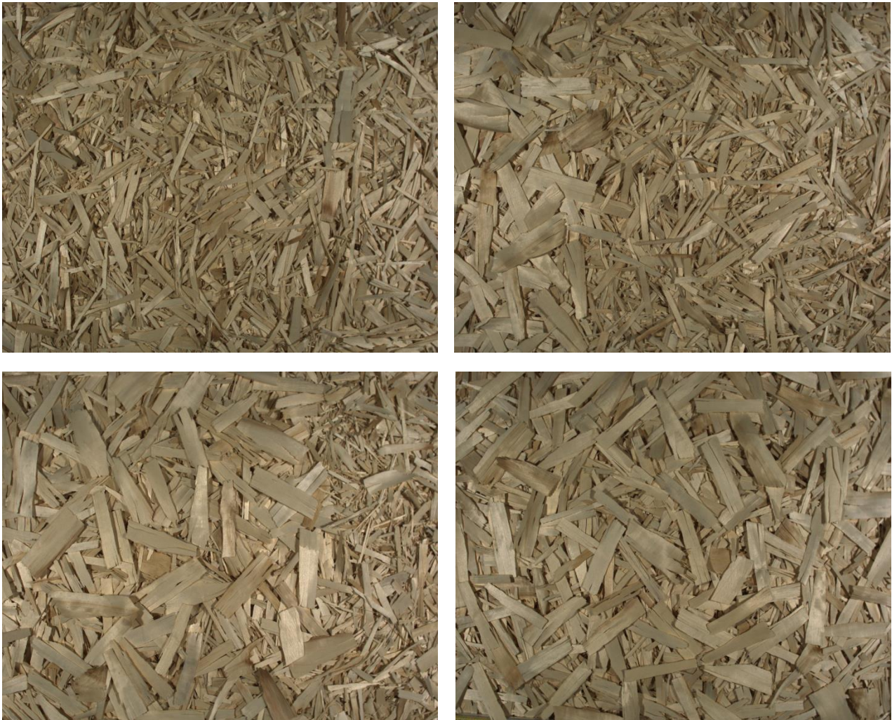
Figure 27 Examples of the images of real wood particles used in the tests. The quality of the strands, according to the target specifications indicated for the project, increases from left to right and from top to bottom.
