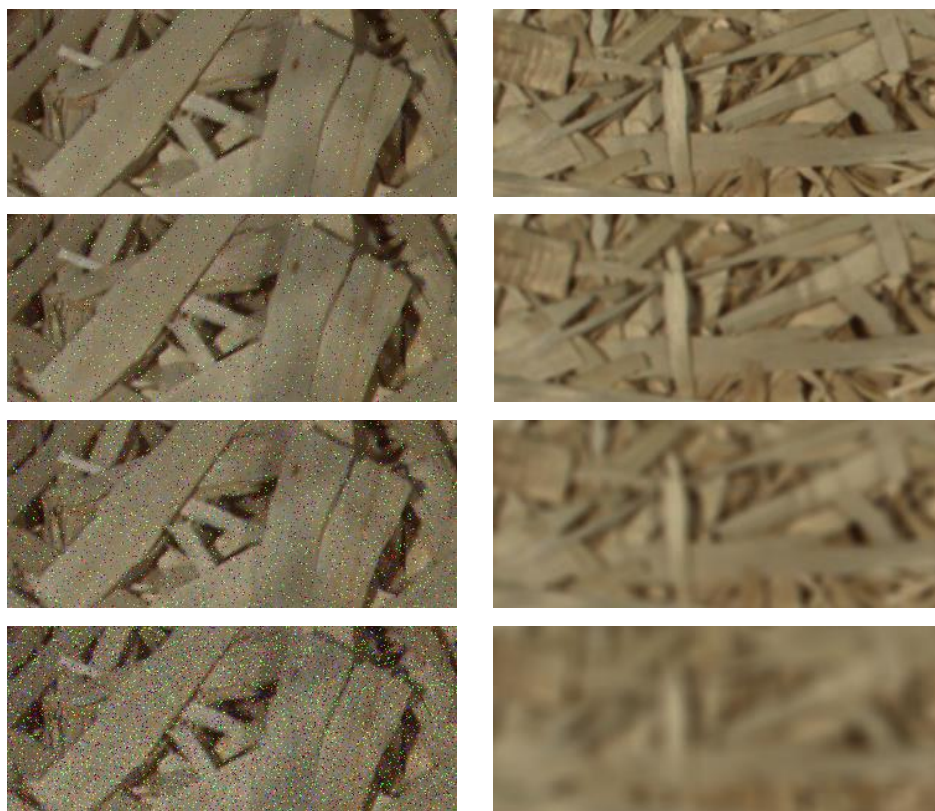
Figure 28 - Examples of the noisy images containing salt and pepper noise, which simulates device noise, (first column) and gaussian blur, which simulates the noise caused by a dirty lens or an out of focus problem, (second column).
