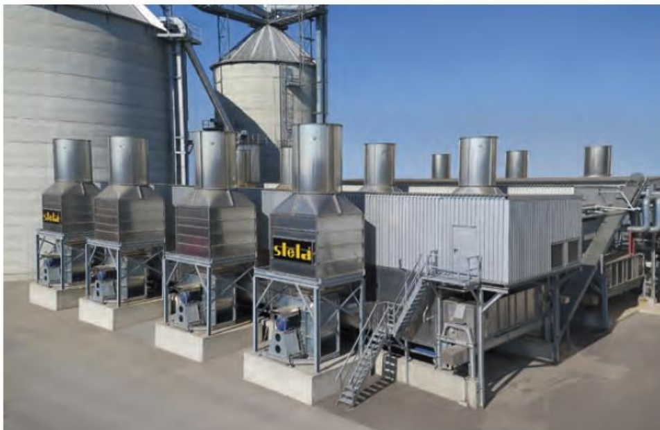
Figure 22 - Stela's low temperature belt dryer
