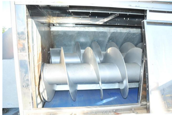
Figure 2 – feeding screws no. 1 (in front) and no. 2 (behind)
