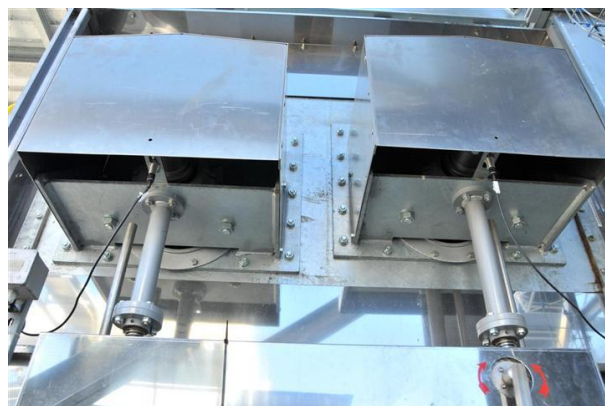
Figure 2 – drives and lifting gears of the distribution screws
