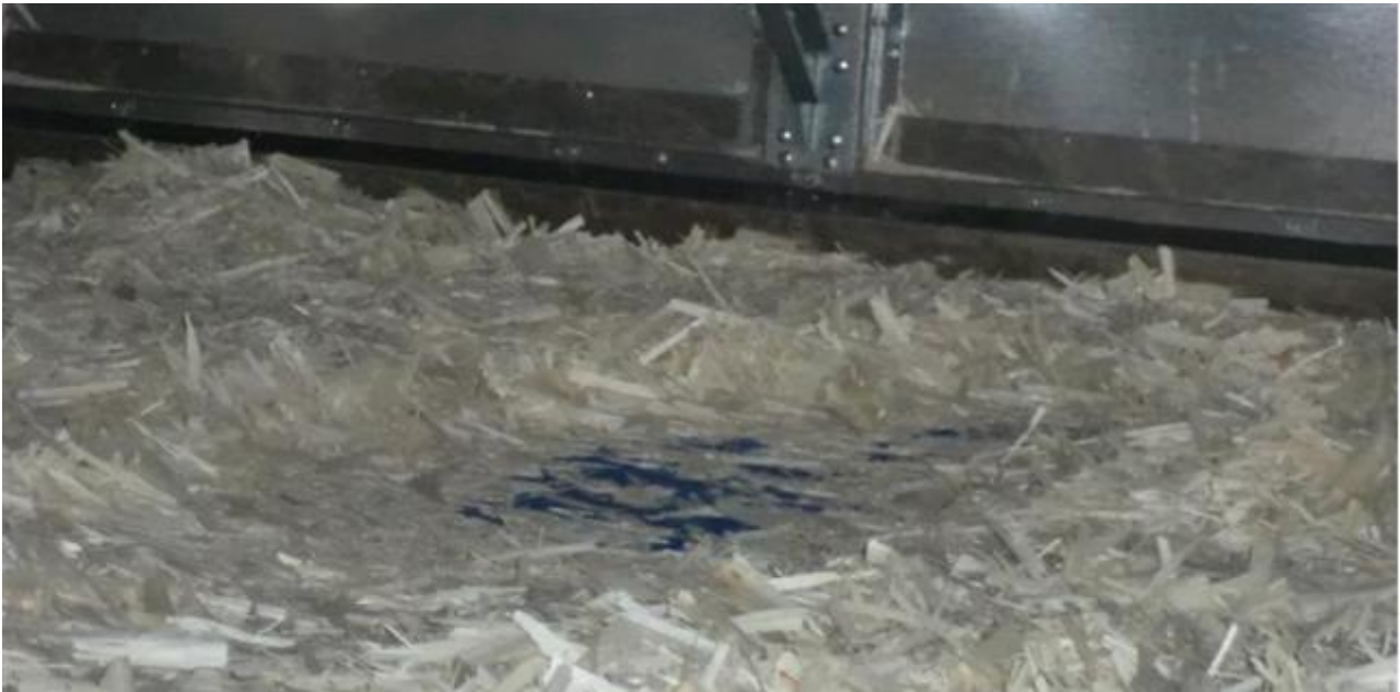
Figure 3 – inadequate product layer on the dryer belt
