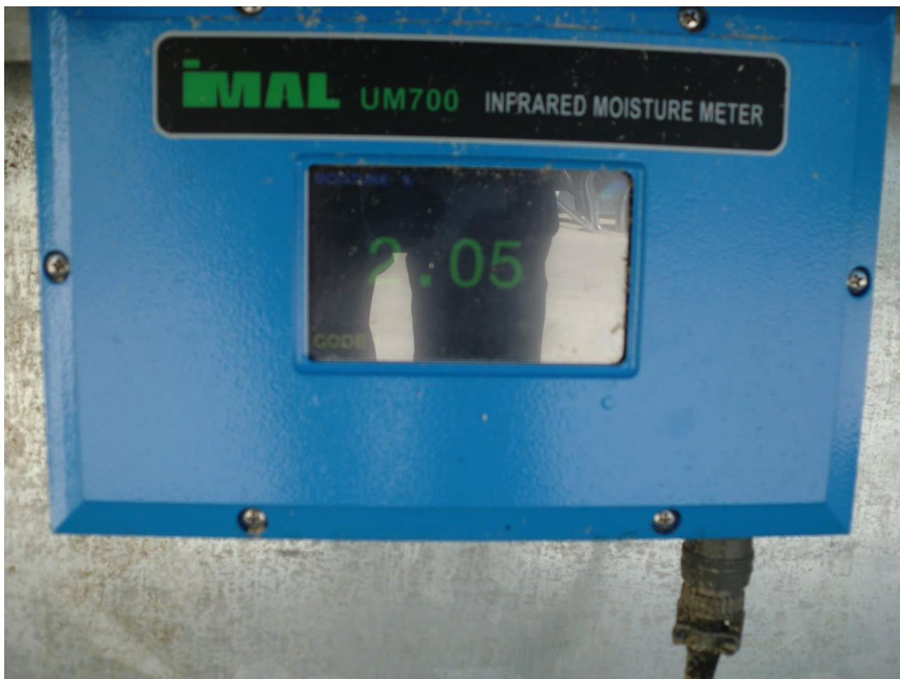
Figure 12 – detail view of the moisture sensor
