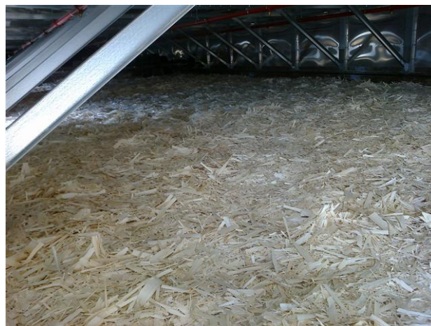
Figure 4 – proper product layer on the dryer belt
