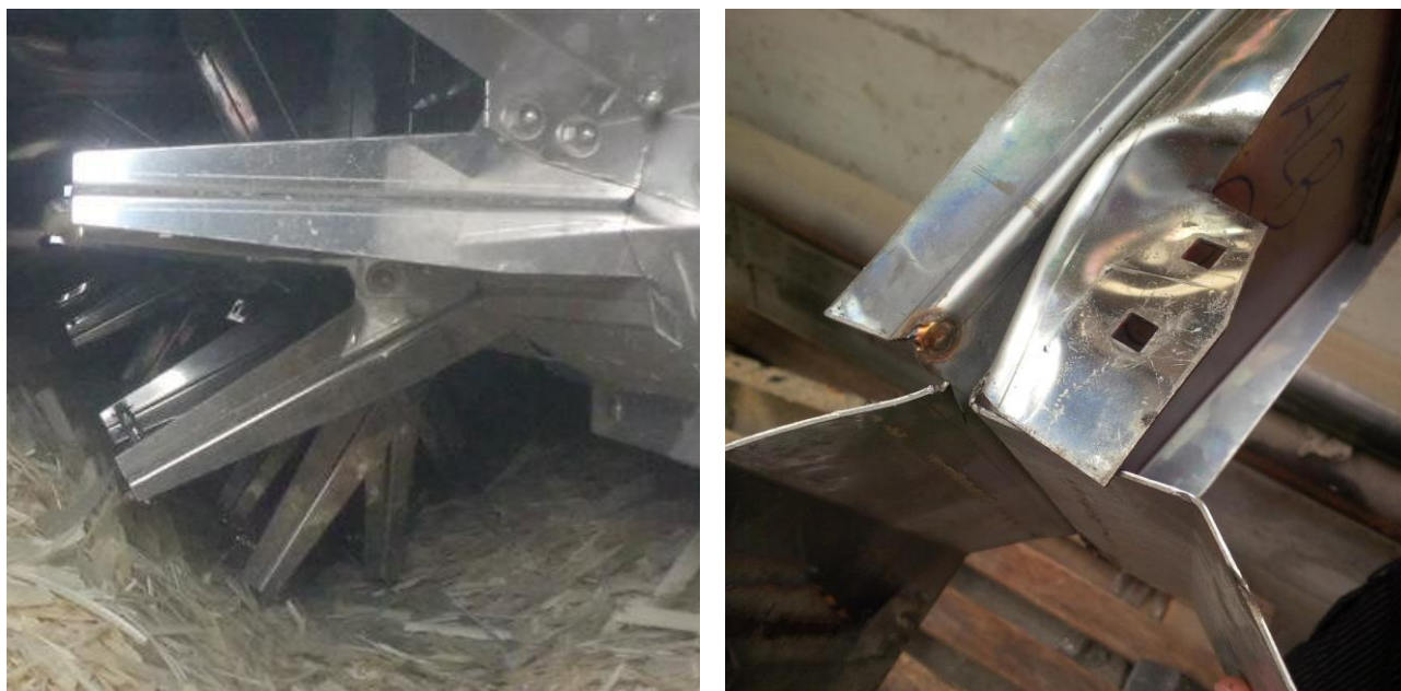
Figure 7: old turning device design (damaged)
