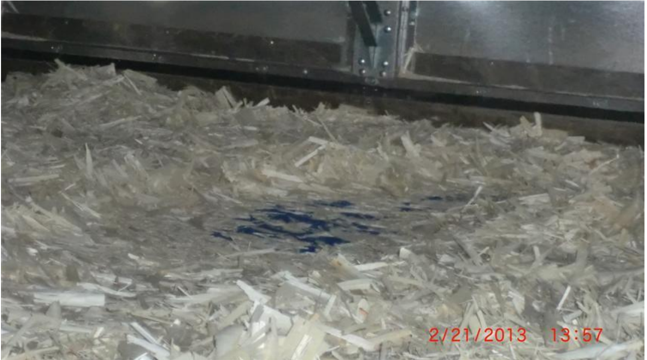
Figure 4: incomplete product layer on the dryer belt
